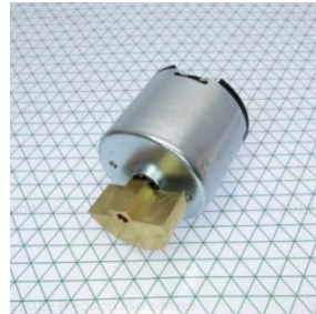
POWER UNIT VIBRATION DATALOGGER WEDGE METAL JACKET TO HOLD DATALOGGER CYLINDRICAL VIBRATION UNIT FINS TO HOLD SAMPLER
